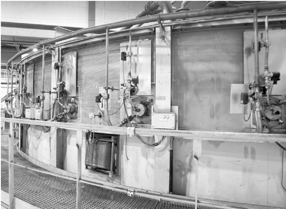
Figure 3: Rotary hearth furnace at Ovako steelworks with simple and compact oxyfuel installations
