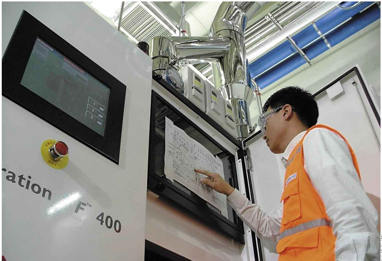
▲ Faster and eco-friendlier: Linde's Generation-F line of on-site fluorine generators allows thin-film PV makers to produce climate-friendly fluorine gas as needed to clean PECVD chambers. The company's joint study with Malibu revealed that fluorine gas has a significantly faster cleaning rate than \text{NF}_3 , which is currently the most commonly used cleaning gas in the industry.
