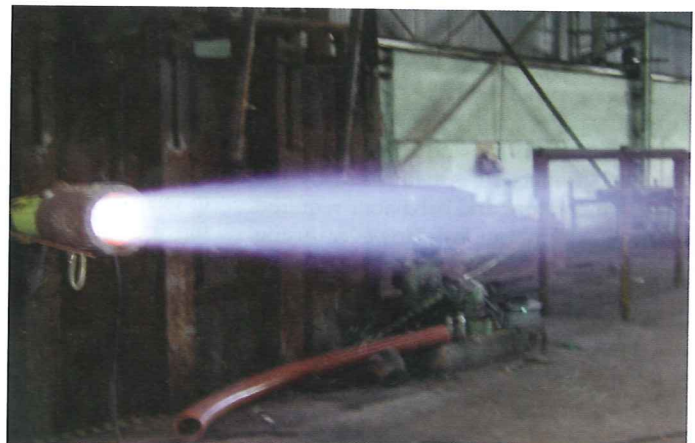
Combustion of blast furnace top gas ( 0.9 \text{ kWh/Nm}^3 , 3.2 \text{ MJ/Nm}^3 ) with air-fuel (left) and oxyfuel (right). With air-fuel the flame is unstable and diffuse, with a bad definition, the flame temperature is 1300^\circ \text{C} and the efficiency is <5\% . In the oxyfuel case the flame is stable and compact with a temperature of 1900^\circ \text{C} and an efficiency of >35\% . The oxyfuel case would correspond to air-fuel combustion of a fuel containing ( 2.1 \text{ kWh/Nm}^3 , 7.7 \text{ MJ/Nm}^3 )
