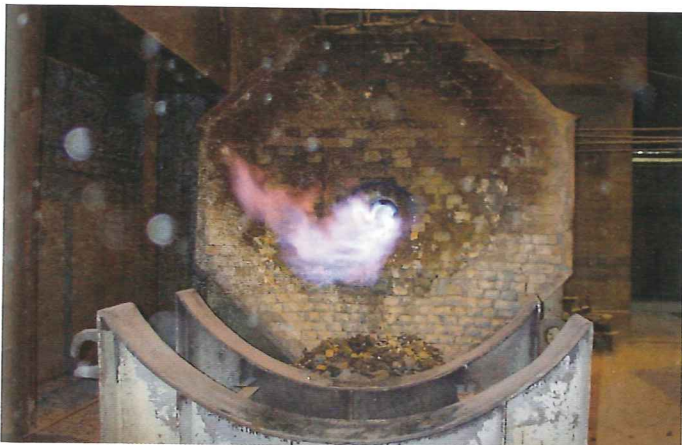
Combustion of blast furnace top gas ( 0.9 \text{ kWh/Nm}^3 , 3.2 \text{ MJ/Nm}^3 ) with air-fuel (left) and oxyfuel (right). With air-fuel the flame is unstable and diffuse, with a bad definition, the flame temperature is 1300^\circ \text{C} and the efficiency is <5\% . In the oxyfuel case the flame is stable and compact with a temperature of 1900^\circ \text{C} and an efficiency of >35\% . The oxyfuel case would correspond to air-fuel combustion of a fuel containing ( 2.1 \text{ kWh/Nm}^3 , 7.7 \text{ MJ/Nm}^3 )
