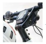
1. Speedometer with light on/off switch. Shows max. speed, trip distance and accumulated distance.
